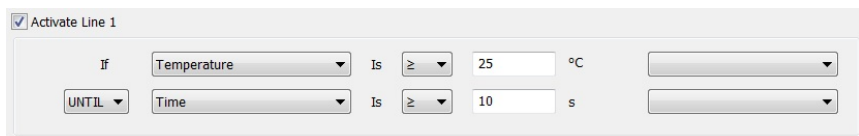
Figure 13 Set time frame logic statement
