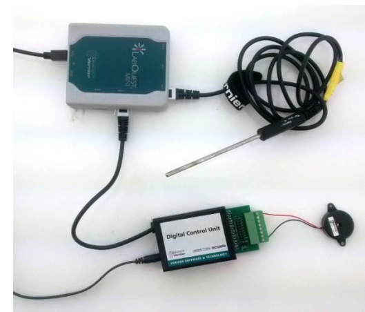
Figure 9 Stainless Steel Temperature sensor, paired with a 5V DC buzzer
