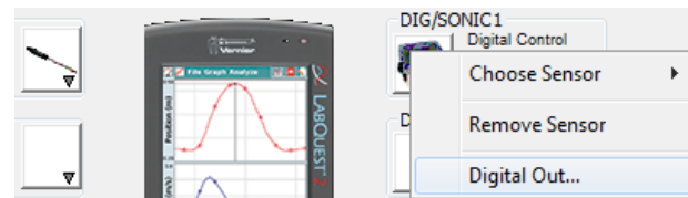
Figure 6 Digital port drop-down menu in Logger Pro
