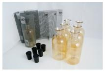
Sensor and a light source to determine the gross and net productivity of an aquatic sample. The screens allow varying amounts of light to pass through the bottles (see below for details) and are designed to be used with the Primary Productivity lab found in several Vernier biology lab manuals.
