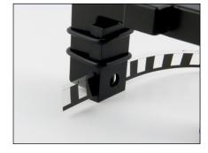
The miniature picket fence will produce very nice motion graphs when dropped through a photogate. The graphs below were all made this way.
