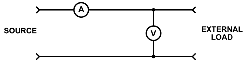
Circuit diagram of how the Vernier Energy Sensor is wired internally
