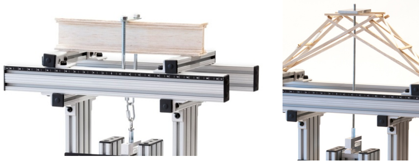
The beam on the left is secured using a U-bolt and quick links while the structure to the right is secured using a threaded rod attached to a metal loading plate.
