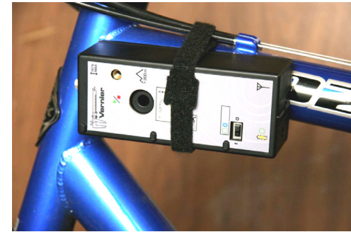
The WDSS on a bicycle for studying acceleration
