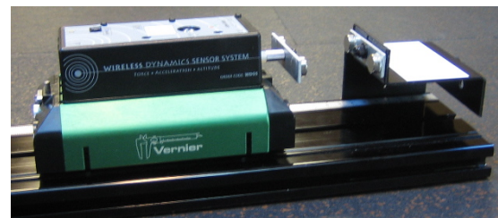
Impulse-momentum setup using Vernier Dynamics Track Adapter (DTA-DFS)
