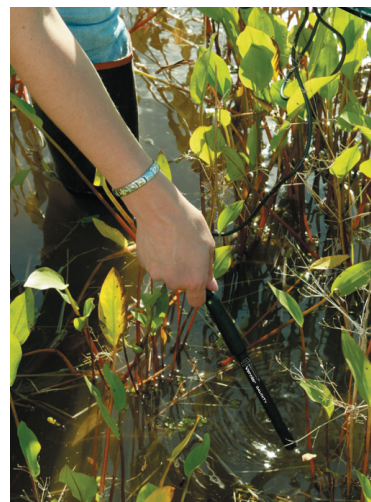
Collecting salinity data of brackish water with the Salinity Sensor
