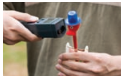
Measuring temperature of the bird with the Infrared Thermometer
