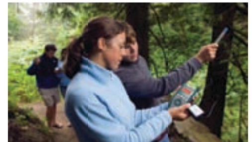
Measuring light level in the forest canopy
