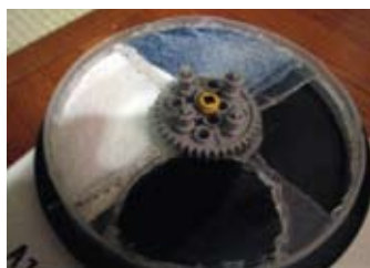
UV pinwheel filter (sunglass lens, cotton shirt, denim, and no filter)
