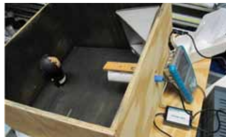
Planet is illuminated from the side while the Light Sensor records reflected light off of varying light and dark patches on the surface of the planet as it rotates.
