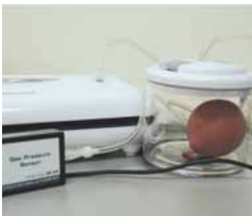
Vacuum sealer with Vernier Gas Pressure Sensor connected
