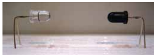
An infrared LED and phototransistor are used to build a photogate.
