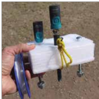
Martin constructed a raft to float Go Wireless Temp and Go Wireless pH away from shore
