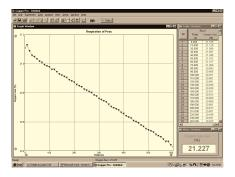
Due to its wide measurement range, the  ${\rm O_2}$  Gas Sensor performs remarkably well for monitoring oxygen concentration during human respiration. This graph illustrates the use of the sensor to monitor the concentration of oxygen gas expired over several trials by a single individual. In each trial, the subject held his breath for a different duration (0, 10, 20, 30, and 40 seconds) before expiring into the sensor. The  ${\rm O_2}$  Gas Sensor will be available in December, 1999.
