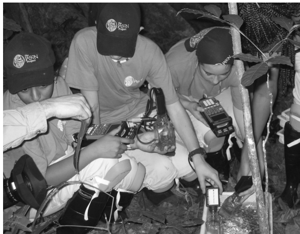
Students using Vernier CO 2 Sensors to study leaf litter on the forest floor. An ice bath was used to vary the temperature of the experiment.
