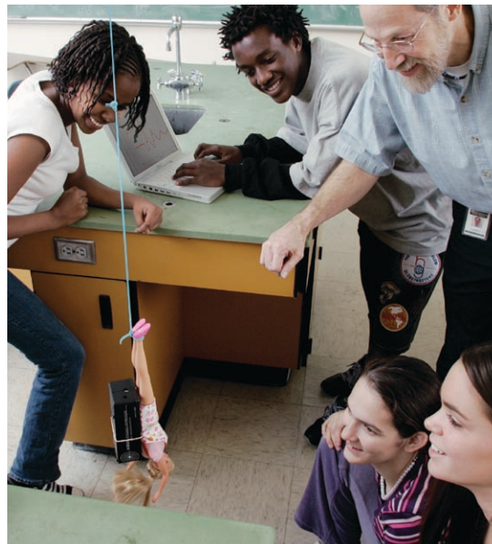
Studying bungee force and acceleration using a Wireless Dynamics Sensor System
