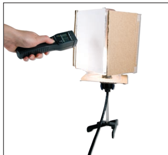
A model house built to test the transfer heat through the walls with the Infrared Thermometer
