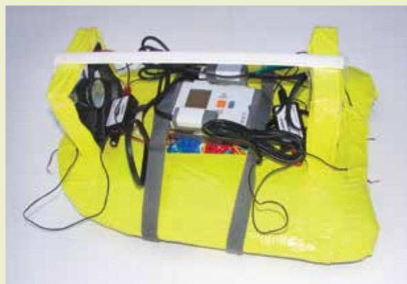
The Aquabot with one LEGO NXT robot, two Vernier NXT Sensor Adapters, and two Vernier Current Probes
