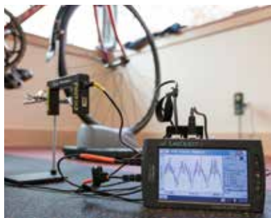
Don't have a goniometer? A photogate can measure cadence and a motion detector pedal position.
