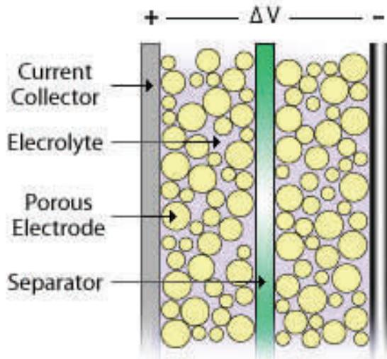
An ultracapacitor can be viewed as two nonreactive porous plates, or collectors, suspended within an electrolyte, with a voltage potential applied across the collectors. In an individual ultracapacitor cell, the applied potential on the positive electrode attracts the negative ions in the electrolyte, while the potential on the negative electrode attracts the positive ions. A dielectric separator between the two electrodes prevents the charge from moving between the two electrodes. (NREL)
