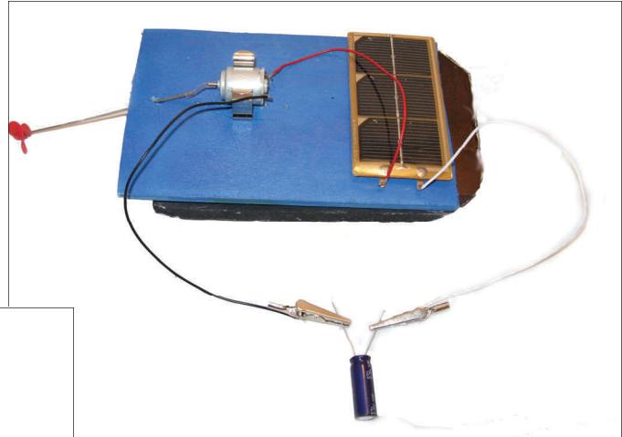
Just connect the supercapacitor in series between the solar panel and the electric motor on your boat (make sure you've connected the right leads). When the panel activates in the sun, part of the electricity created will
