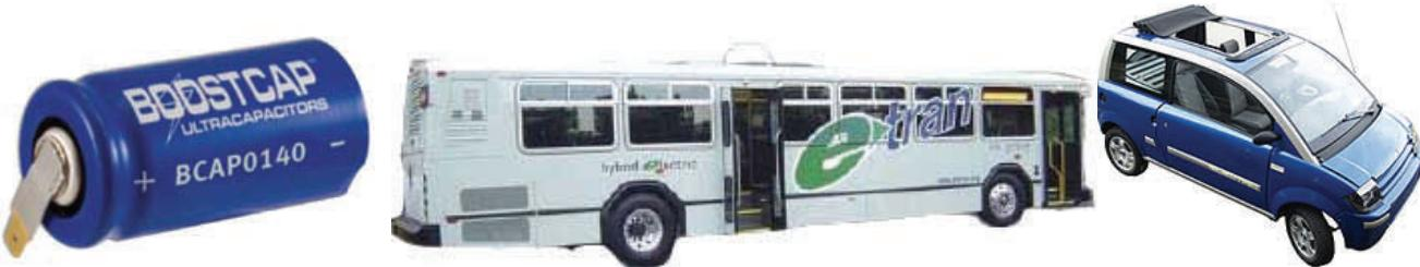
*Larger supercapacitors are used in hybrid-electric vehicles. They are charged when the vehicles brake, and discharged to enhance acceleration.*
